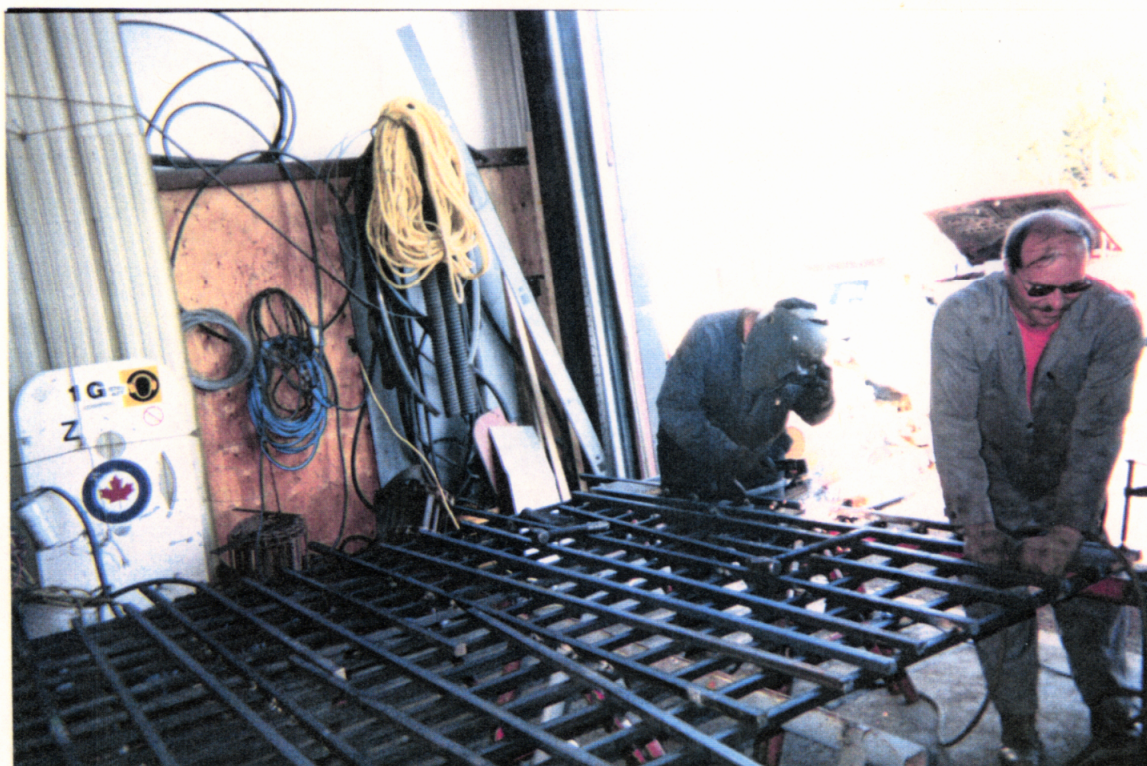
PHOTO E-2: Shop fabrication of steel grate for No. 2 Shaft closure.
