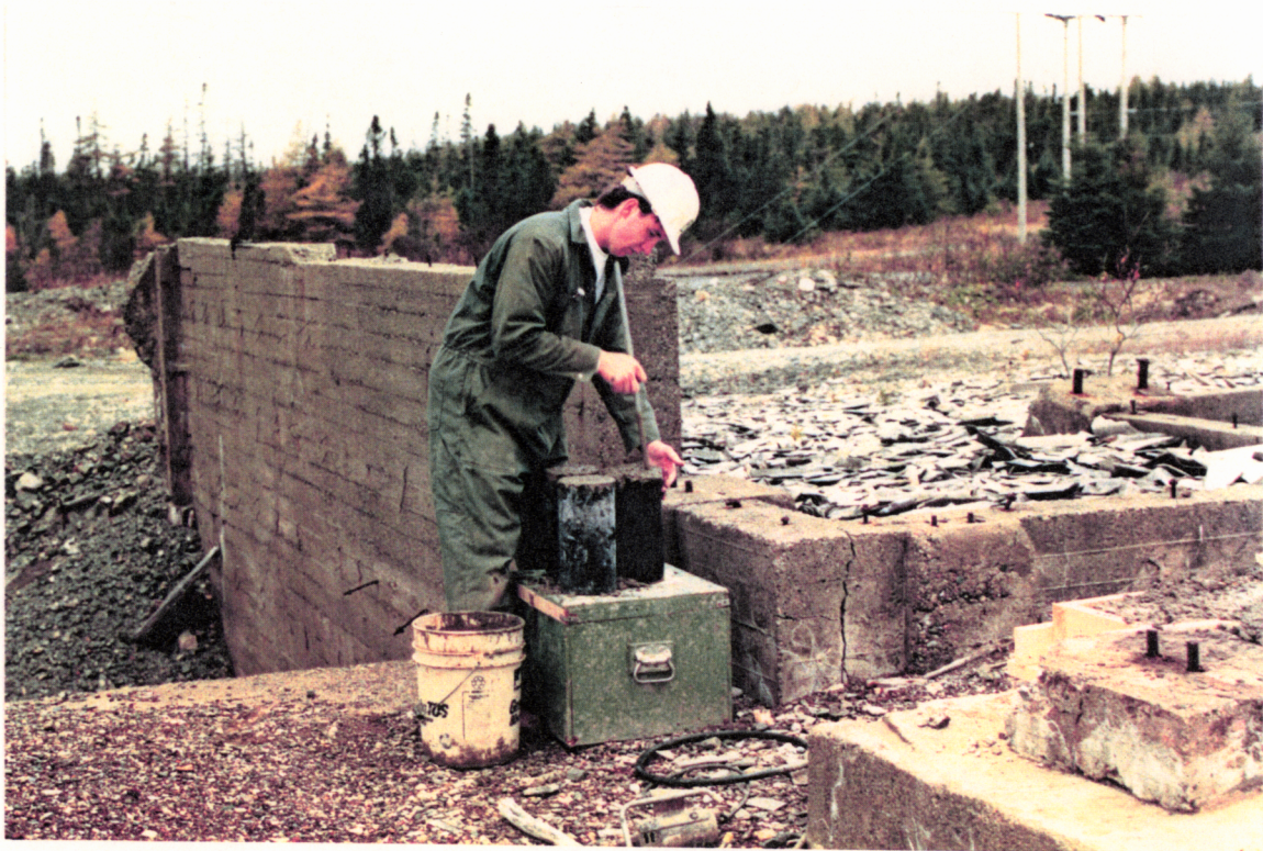
PHOTO NO. H-8: Obtaining concrete test cylinders to determine compressive strength of concrete.
