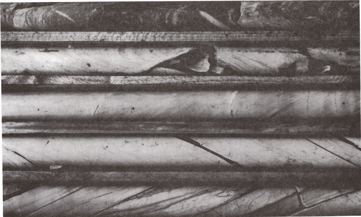
Figure 5. Photograph of diamond-drill core from hole KA-2 (box #14) at the Stirling deposit showing intense alteration of the host rock due to replacement by quartz-talc-carbonate rock. Note the well-developed fabric in the rocks and also late-stage quartz veins with alteration halos in the right end of the centre piece of core. Width of the core is ca. 3.5 cm.
