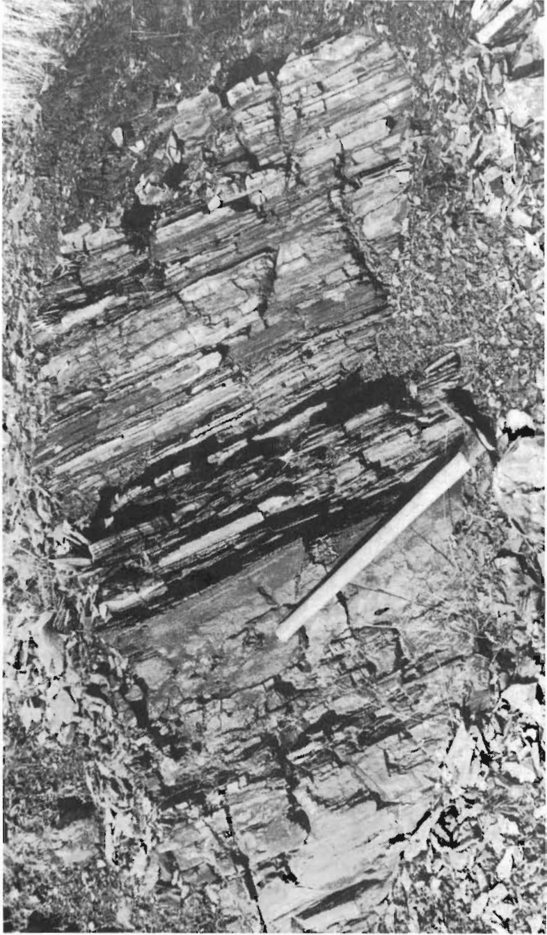
Thin bedded Canso shales in cut on Highway No. 5, Port Hastings, Nova Scotia.
