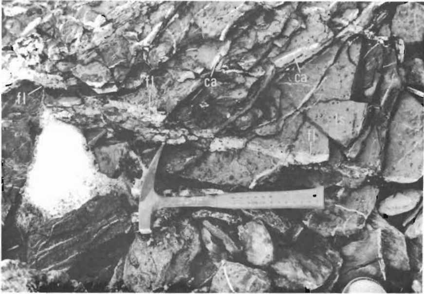
Figure 173 - Detter Creek. Fluorite veins in thinly laminated limestone (lower Windsor Group), fl - fluorite, ca - calcite.
