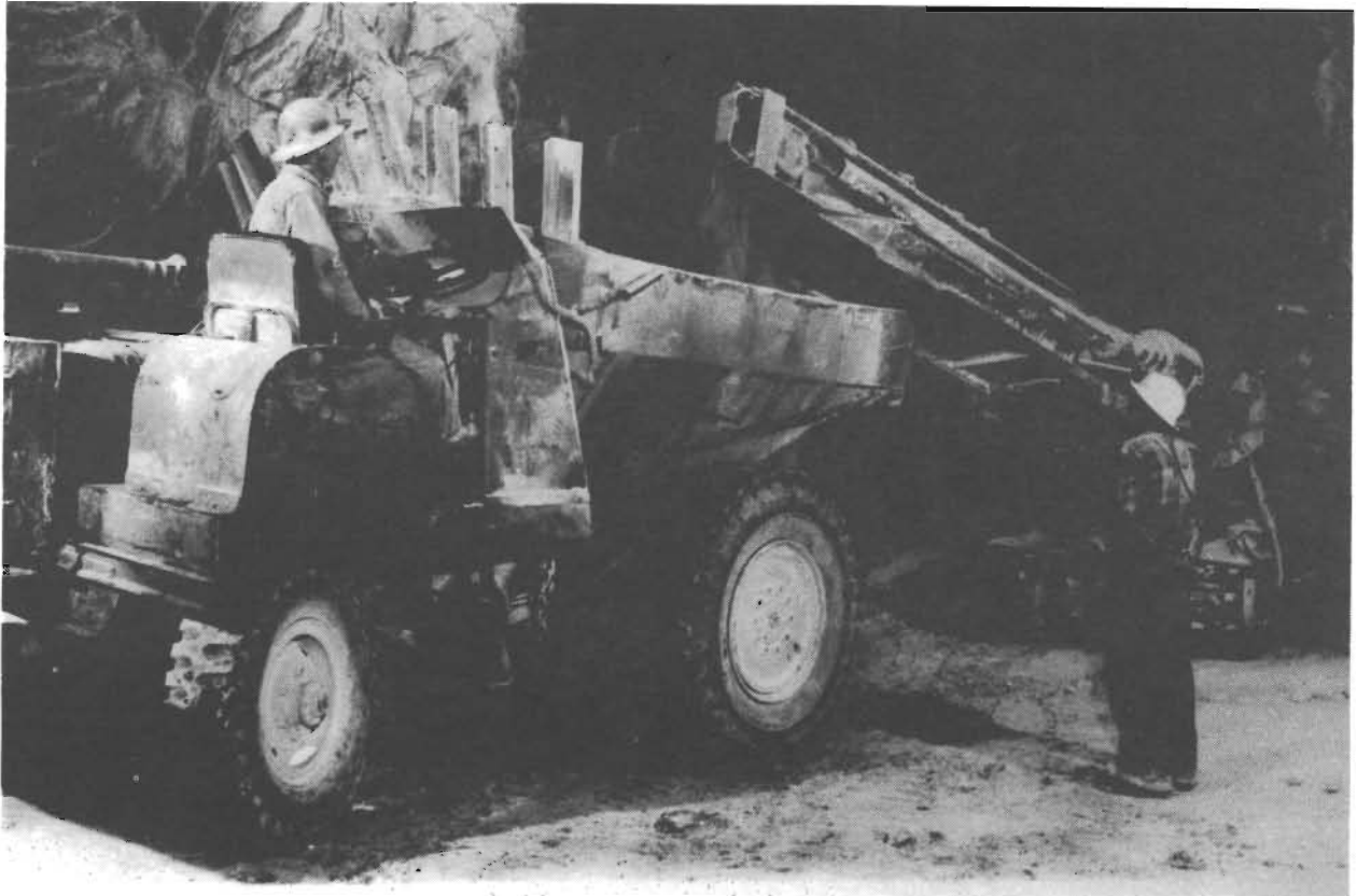
Loading salt into haulage trucks, Pugwash Mine (NSIS).
