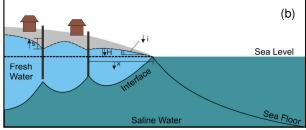
Figure 3. Conceptual illustration showing how vulnerability to SWI impacts can increase according to the Ghyben-Herzberg relationship. In (b), the water supply wells are at greater risk due to lower freshwater head above sea level (H) as a consequence of their closer position to the coast, a lower hydraulic gradient (i) and increased drawdown (s).
