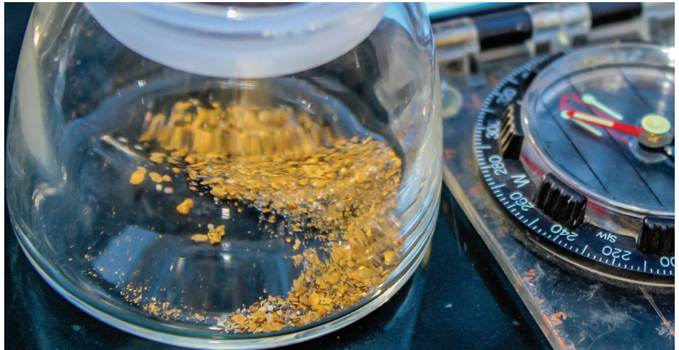
Figure 2. Vial of gold grains obtained from crushing a 5 gallon bucket full of quartz collected from waste piles at the Pockwock Au Prospect.
