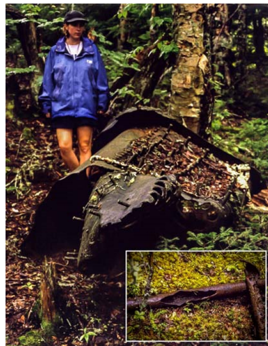
Figure 1. (L) Air photo showing the location of the Gold Lake Mine and position of the 1897 boiler accident relative to the mine workings. Figure 2. (R) Photo of the boiler firebox showing extensive damage. The inset is a photo of a ruptured pipe from the boiler, showing clear evidence of the steam explosion.
