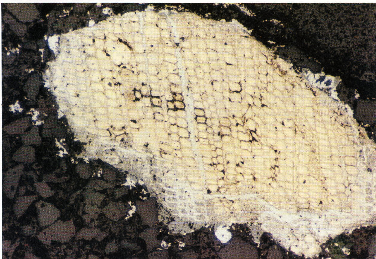
Pyrite, sphalerite and galena, in coalified plant fragment, in sandstone.
