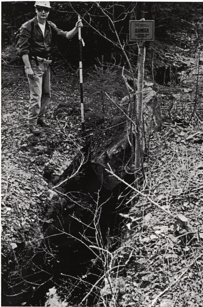
Figure 6: A water filled stope along a gold vein which has partially caved through to surface.
