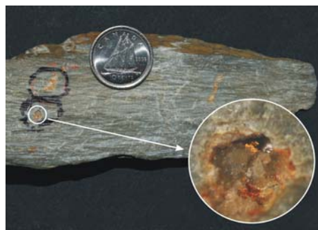
Figure 2. Sample of silicified and sericitized argillite from the Schoolhouse Brook Au occurrence with veinlets and vugs of quartz-sericite containing visible gold (see inset photo).
