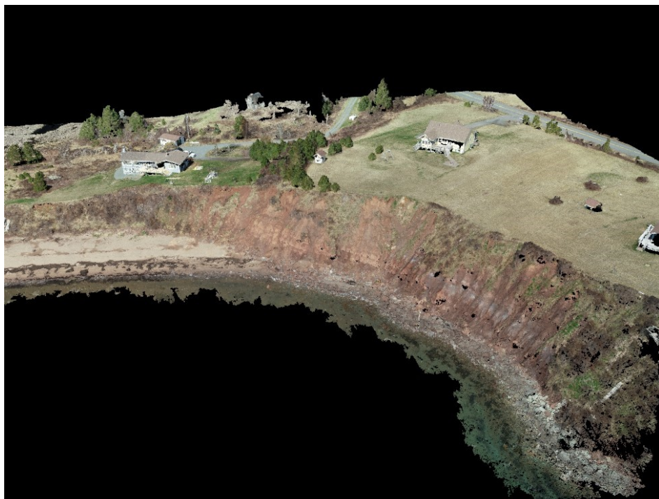
Point cloud image from the first drone survey near Antigonish (250 points per m 2 ).
