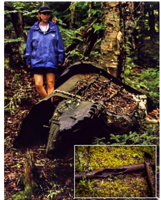
Figure 1. (L) Air photo showing the location of the Gold Lake Mine and position of the 1897 boiler accident relative to the mine workings. Figure 2. (R) Photo of the boiler firebox showing extensive damage. The inset is a photo of a ruptured pipe from the boiler, showing clear evidence of the steam explosion.
