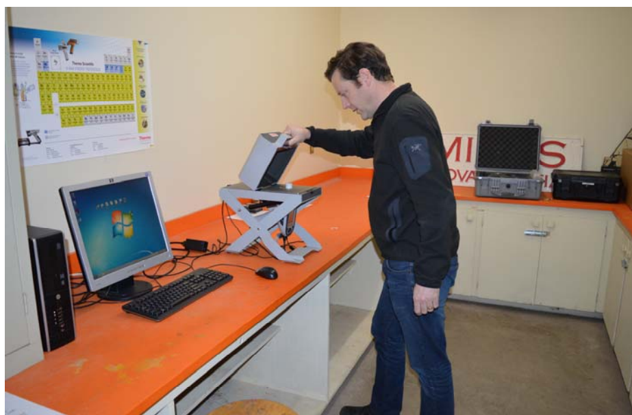
The DNR Core Library in Stellarton is home to a new X-ray Fluorescence device, shown above, which allows prospectors to obtain immediate geochemical analyses.
