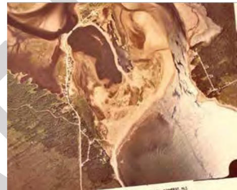
Figure 1: 1954 (top) and 1974 (bottom) aerial images of Rainbow Haven Beach, showing the sedimentation of the western seaward shore. Early maps show that the original entrance channel into Cole Harbour passed through the historical dyke bridge, while the current entrance channel to the east is newly formed (Davies et al 2011).
