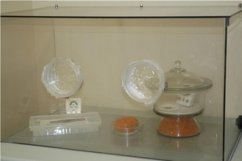
Fig. 4 Experimental desiccation system involving two chambers to reduce humidity levels
