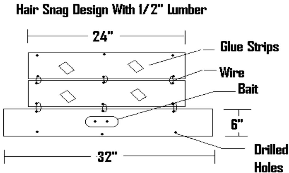
**Figure 1.** Hair snag design with three boards wired together
