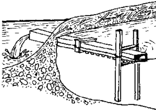
Beaver pipes have been constructed of wood, four-, six-, or eight-inch (10-, 15-, or 20 cm) diameter sewage pipe, corrugated drainage pipe, old metal culverts and other suitable materials. This system works on the principle that beaver build dams in
