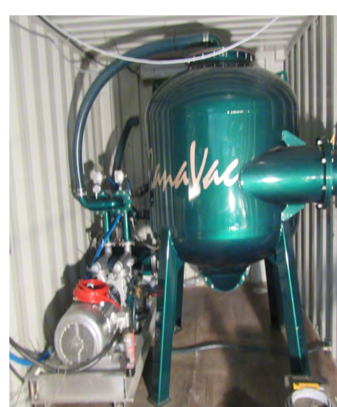
CURRENT CANAVAC FISH TRANSFER SYSTEM
