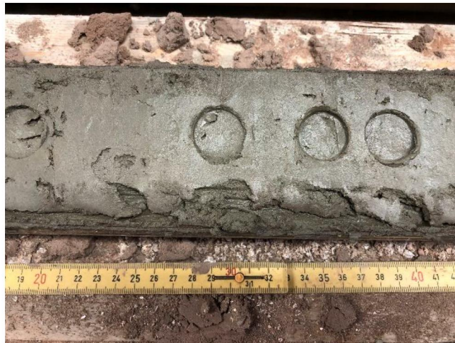
Figure 5.2.2 – Vibracore sample from VC20 composed of silt.
