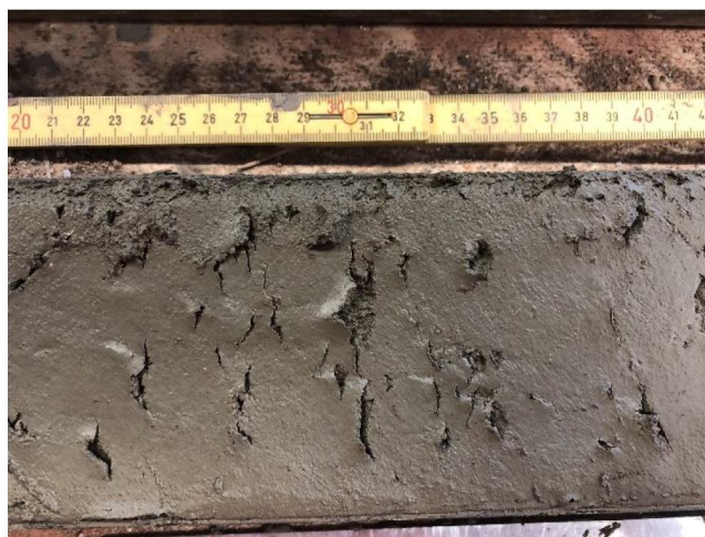
Figure 5.2.3 – Vibracore sample from VC53 composed of silt.
