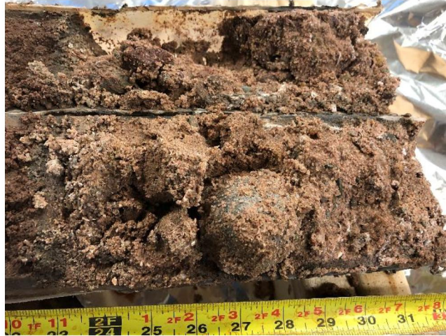
Figure 5.2.1 – Vibracore sample from VC1 composed of coarse sand and gravel.
