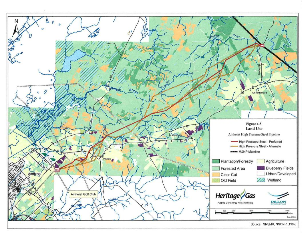
Effects on agricultural productivity can be caused by: construction workspace requirements; access for construction; dust generation onto adjacent sensitive crops; and effects on livestock from equipment noise and blasting. Where agricultural lands are excavated or used by heavy equipment, soils may be mixed or compacted, which reduces crop productivity.
