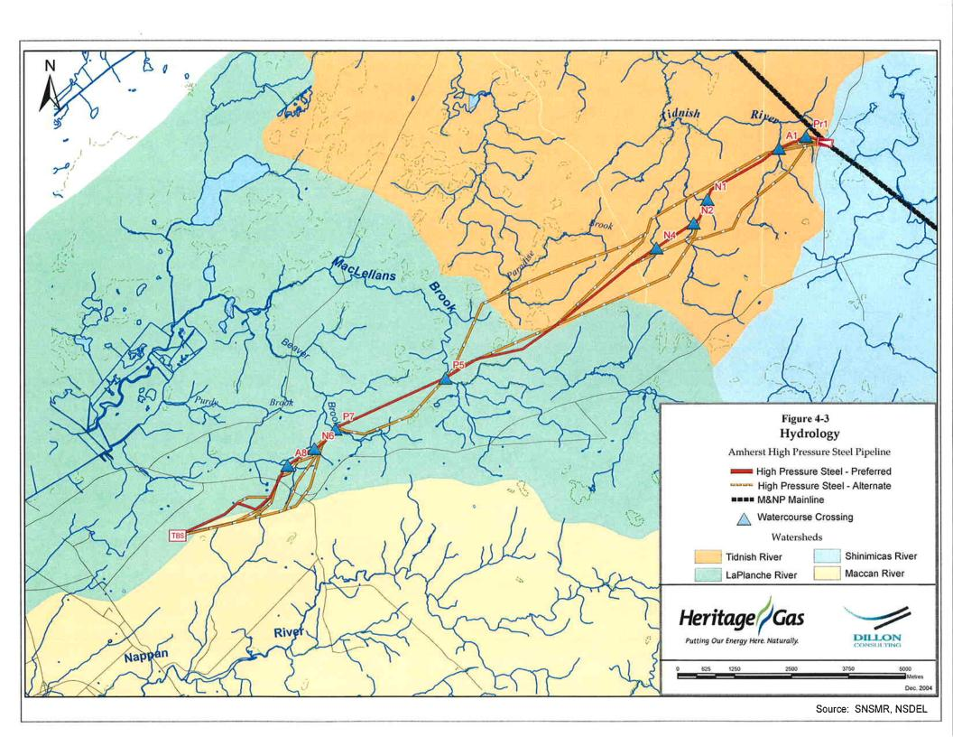
Sensitivity of fish habitat is a key criterion in selecting a watercourse crossing method. The use of isolated crossing techniques (i.e., dry crossing methods and directional drilling), selection of an appropriate time for construction of the crossing (June to September), and standard environmental protection practices throughout the project emphasize protection of fish and fish habitat and erosion and sediment control. No wet crossings of watercourses are proposed for this project.
