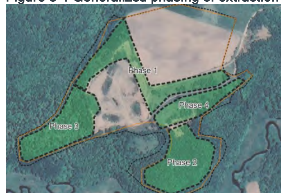
Figure 5-1 Generalized phasing of extraction
