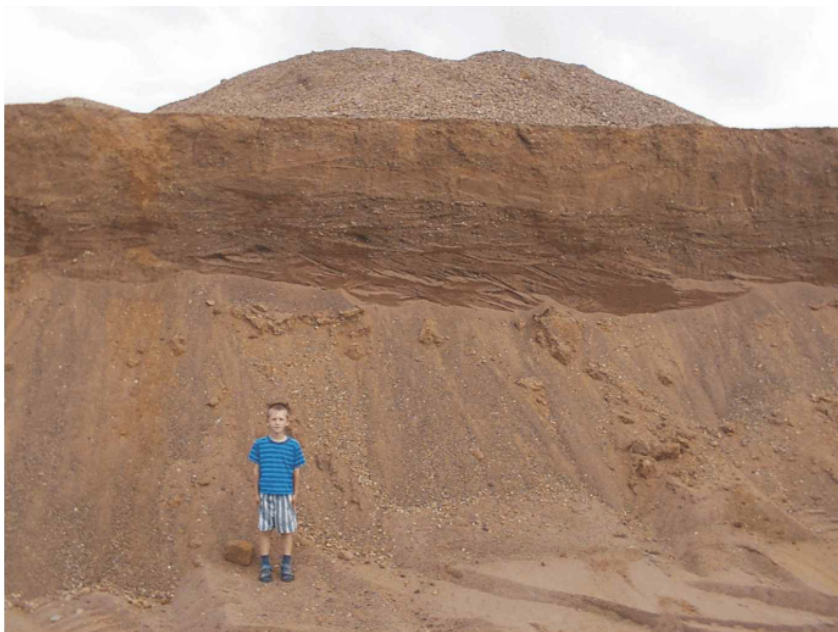
Figure 6. Pit exposure in northwest quarter of the property. The sediment is glacio-fluvial outwash and is moderately to well-sorted with high conductivity. These deposits tend to be rarely thicker than 10 m and laterally continuity can be highly variable. Lodgement till and/or glaciolacustrine sediment (both with low conductivities) most often underlies these deposits.
