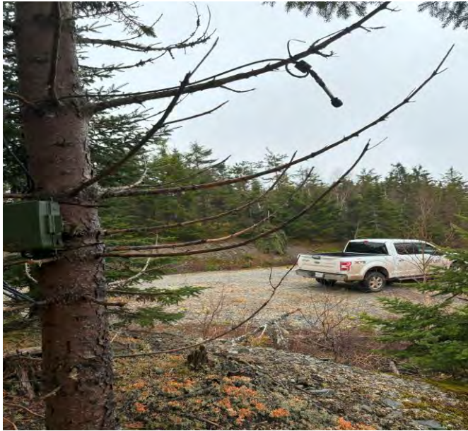
Photo 5: Bat 3 microphone installed on tree branch
