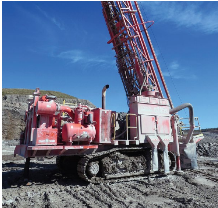
Photo.B.1.5 Production drill used to drill holes for blasting process.
