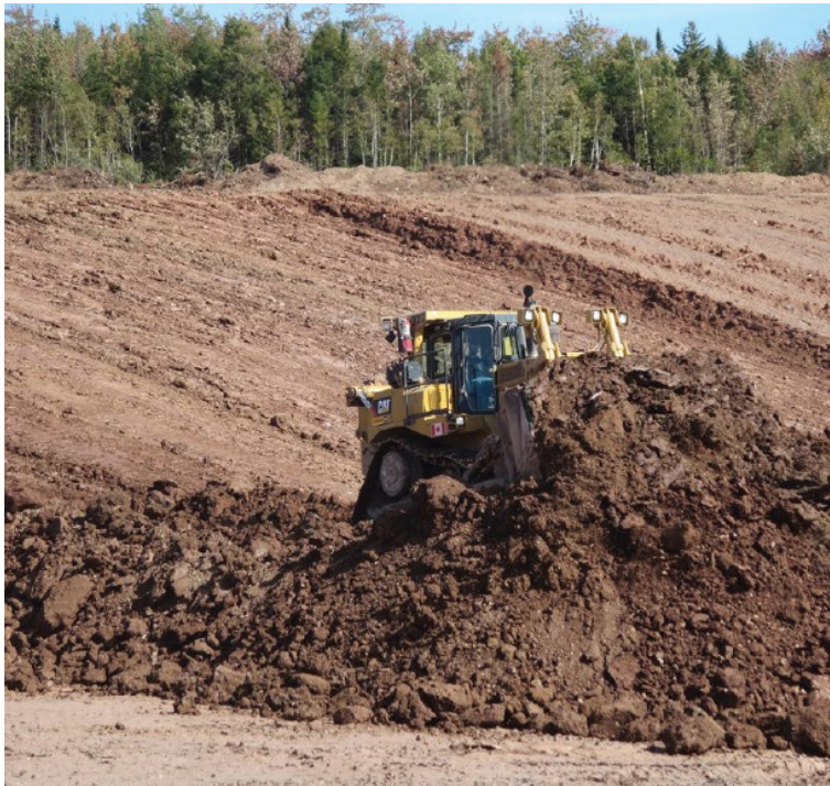
Photo.B.1.7 Bulldozer moving mud to uncover gypsum rock.
