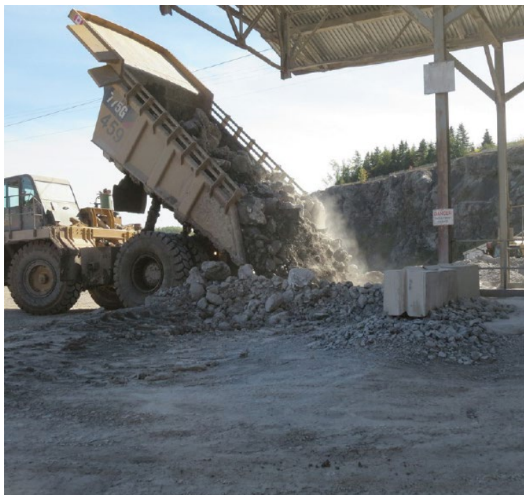
Photo.B.1.8 70-ton truck dumping gypsum ore at the crusher for processing.
