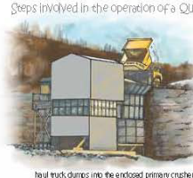
haul truck dumps into the enclosed primary crusher
