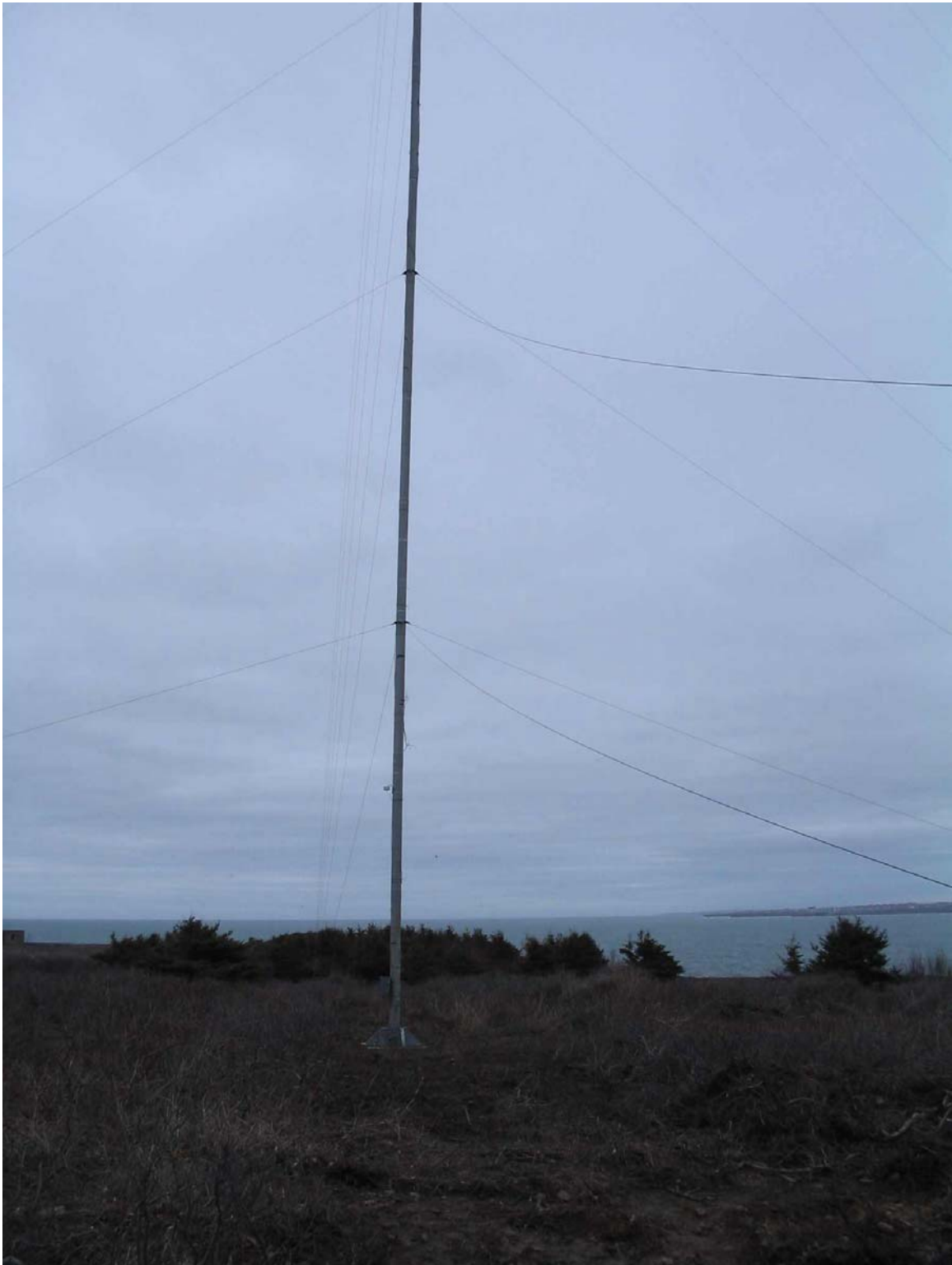
Figure 7: The base of the anemometer tower showing guy wires and looking towards E and the end of the peninsula.
