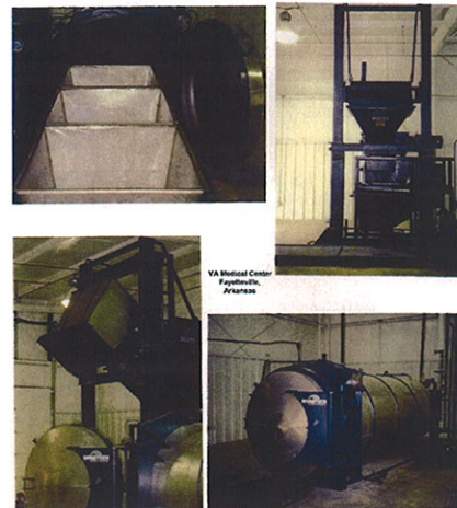
On-site hospital operation depicting: Aluminum bins, shredder, bin dumper and Bondtech's autoclave.
