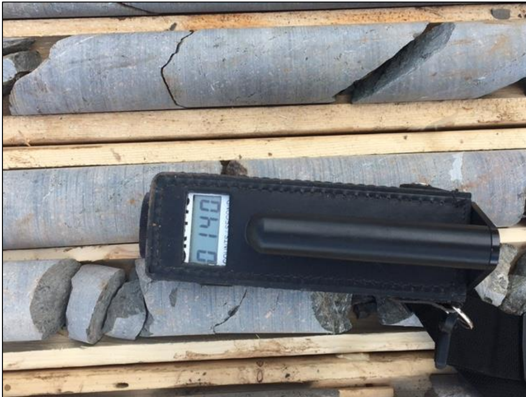
Figure 7-2: Area of higher background core (140 cps) in hole BH
