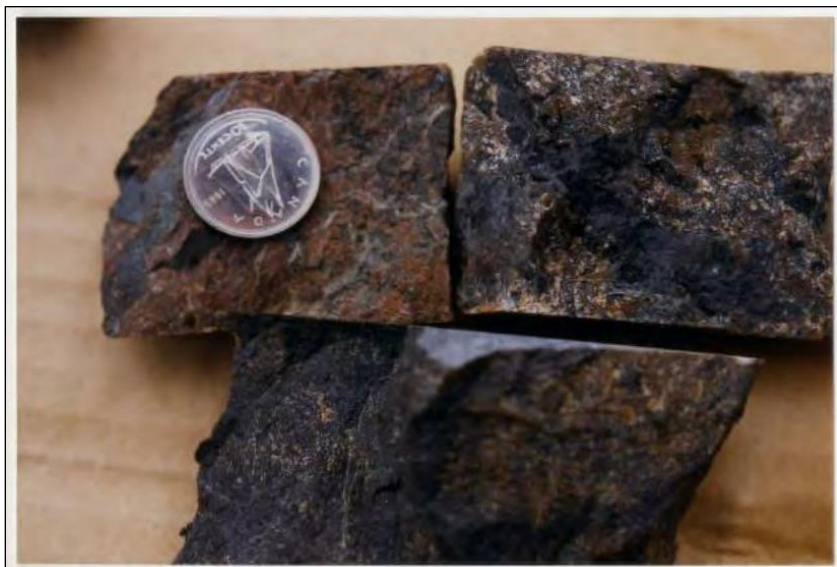
Figure 3-2: Drill core samples of brecciated rhyolite with dull metallic grey to black pitchblende (uranium ore mineralization) from Gulf Minerals DDH DF-32 (Taken from Gower, 1988)
