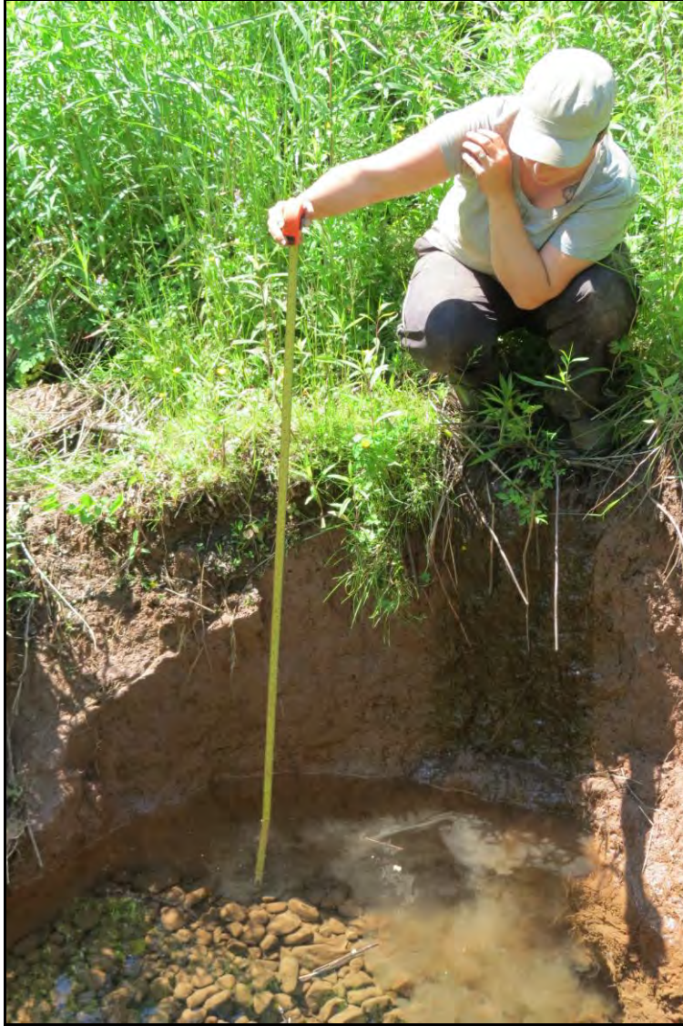
PLATE 22: Thickness of sediment and underlying cobble layer at a creek bed on the east side of Middle River, facing east. June 18, 2013
