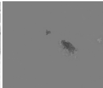
Composite of two images showing ship and false echo.
