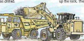
Haul truck is filled by a face loader at the muck pile.
