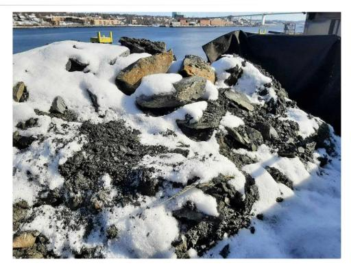
Photo 1. Sediment from the Upper Layer, collected via dredging as part of the Pilot Study
