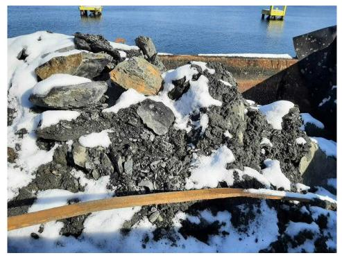
Photo 2. Sediment from the Upper Layer, collected via dredging as part of the Pilot Study
