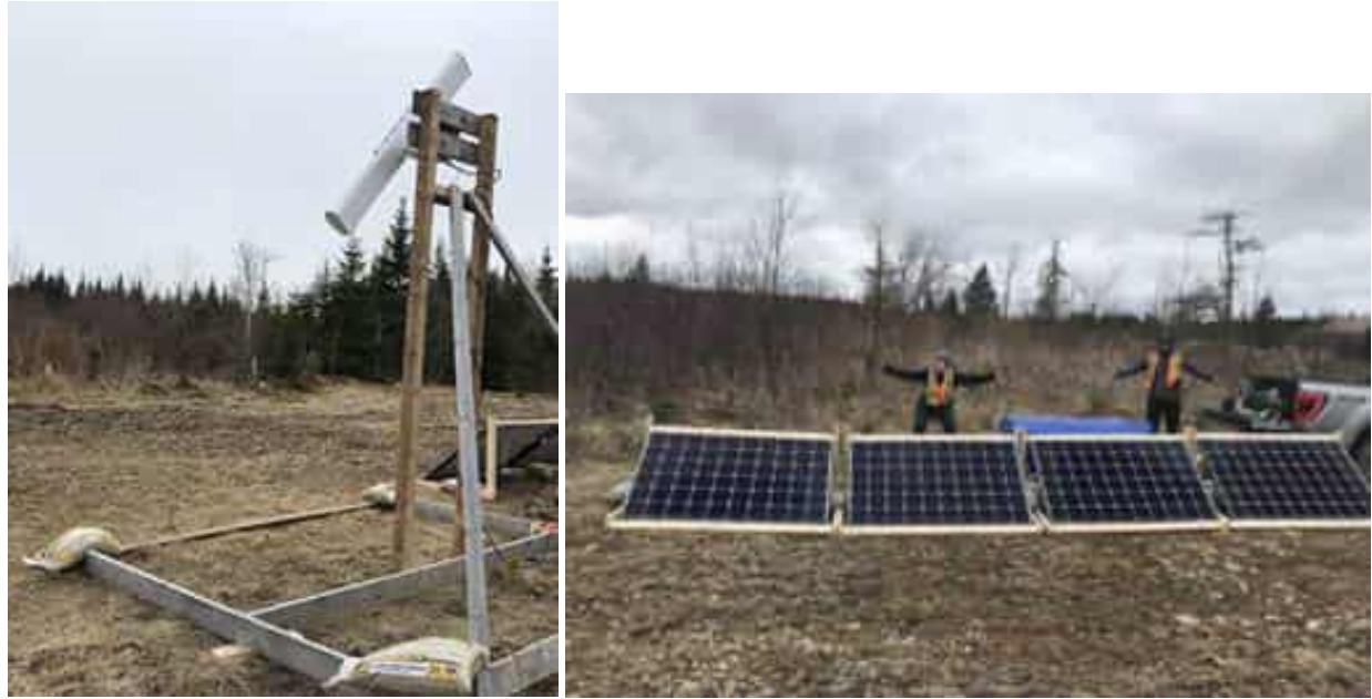
Figure 2.1 Photographs of Radar Setup Including Support Structure, Solar Panels and the Furuno 1962 Marine Radar Antenna
