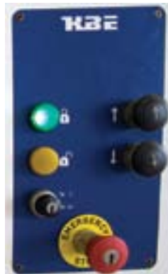
Emergency Stop Button
