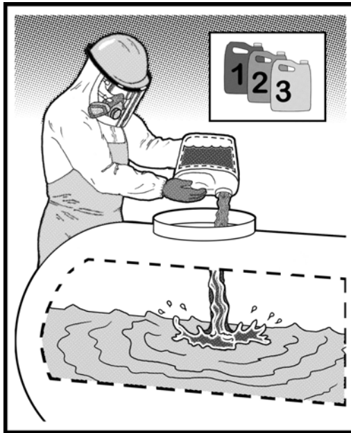
Figure 5-7: Triple rinse plastic or glass pesticide containers.
