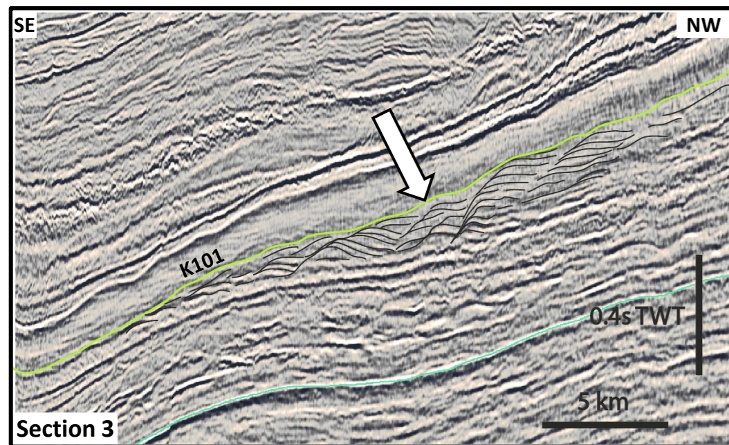
Section 3 Seismic examples of climbing-up antidunes on the Banquereau paleoslope. Such organization could be explained by the reworking of underlying strata by downcascading underwater density currents.
