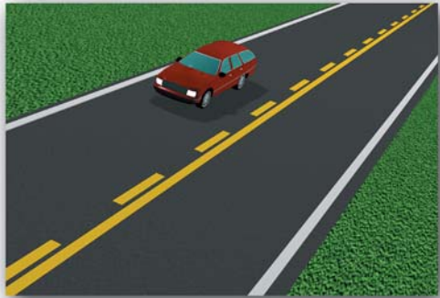
Broken Centre Line with Solid Line
