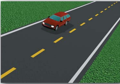
Broken Centre Line
