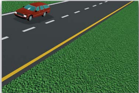
Left Edge Solid Yellow Line on a Divided Highway
