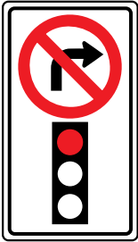
No right turn on red signal. Wait for green light before making a right turn
