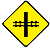
This warning sign is usually posted in advance of the Railway Crossbuck sign
