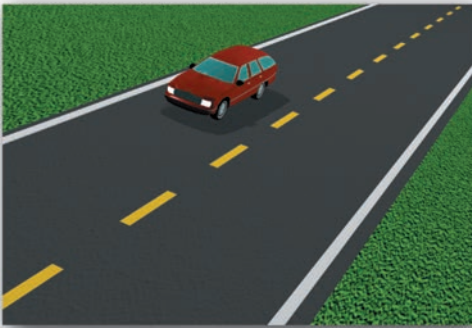
Broken Centre Line
