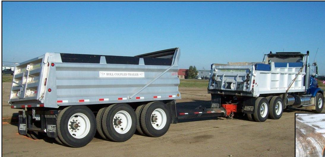
Pony trailer applications for the Wolf roll-coupling hitch include log haul, flat deck, tanker, and dump configured combinations. More information on this technology and other roll-coupling products is available on our website: [www.wolftrailer.com](http://www.wolftrailer.com).
