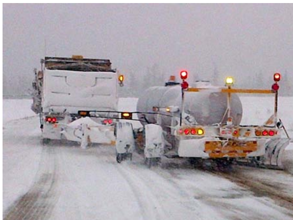
Rear view of unit in working position. Vehicles cannot pass a working tow plow on a four-lane divided highway.
