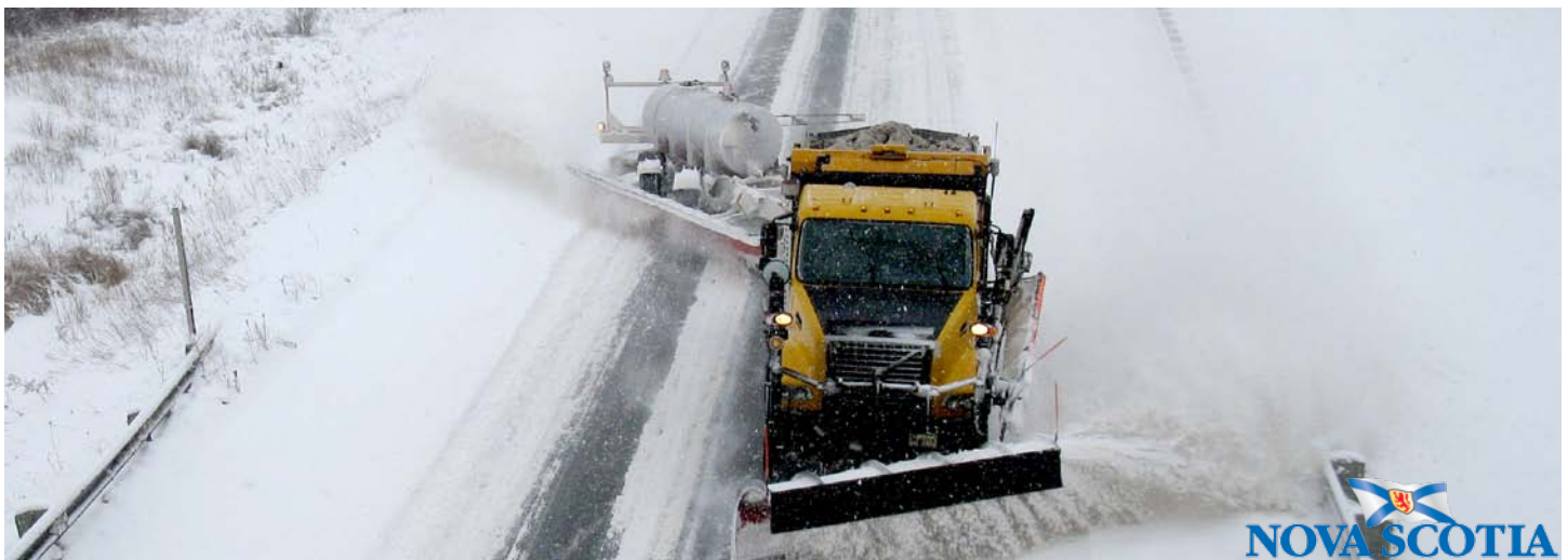
Rear view of unit in working position. Vehicles cannot pass a working tow plow on a four-lane divided highway.
