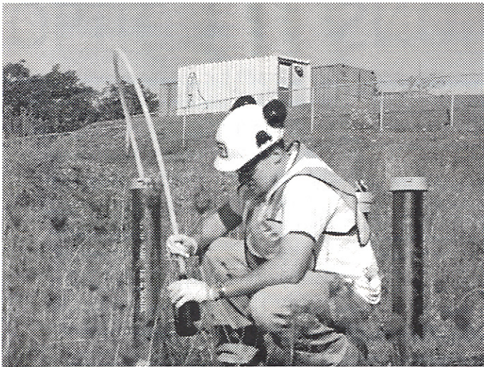
Caption: Jacques Whitford representative taking sample from groundwater monitoring well.
