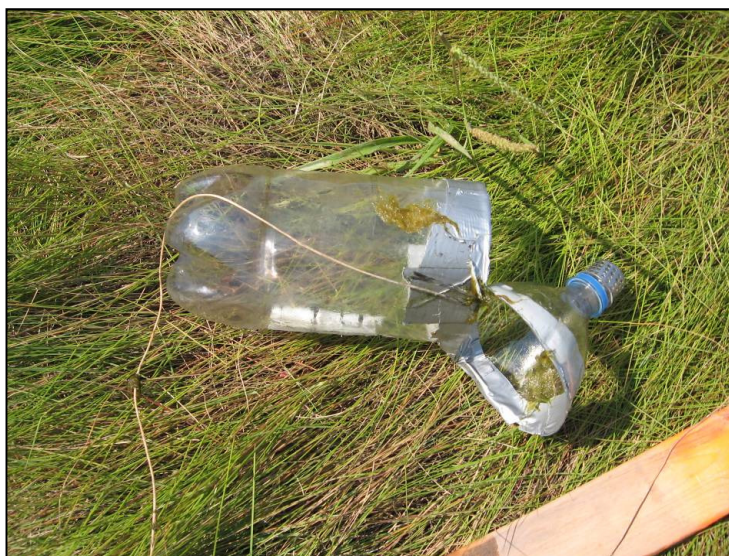
Figure 19 Invertebrate Activity Trap (IAT). Photograph by T. Bowron 2007.
