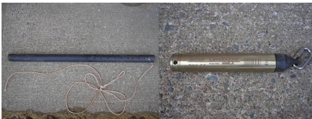
Figure 9 Solinst Model 3001 Levellogger Gold and still well. Photograph by N. Neatt, January 2008.
