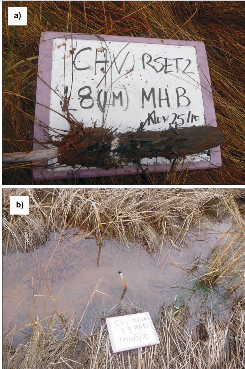
Figure 43 Marker horizon B at a) RSET-02 transect 8 in the low marsh on November 25, 2010 showing 5.48 cm of sediment accretion since 2006 and b) RSET-04 in water on November 25, 2010.
