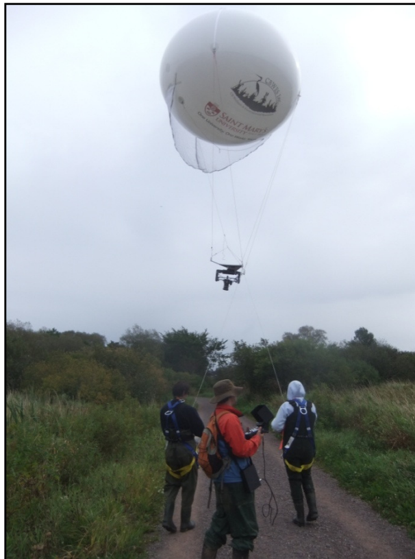
Figure 6 Small format aerial photographic platform using helium filled blimp with a suspended camera system. Photograph taken at Antigonish site by T. Bowron, September 2010.
