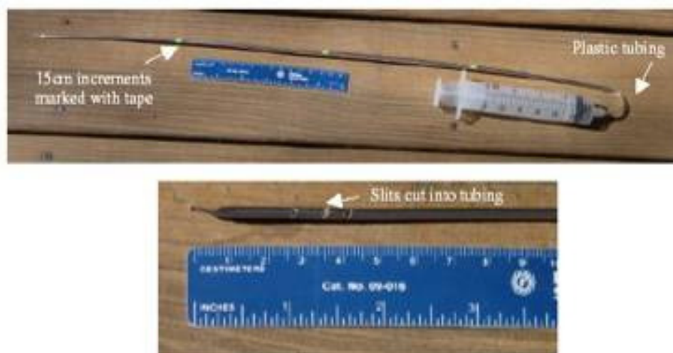
Figure 10 Photograph of a soil probe (sipper) used to take an interstitial pore water samples to test for pore water salinity (Roman et al. 2001).
