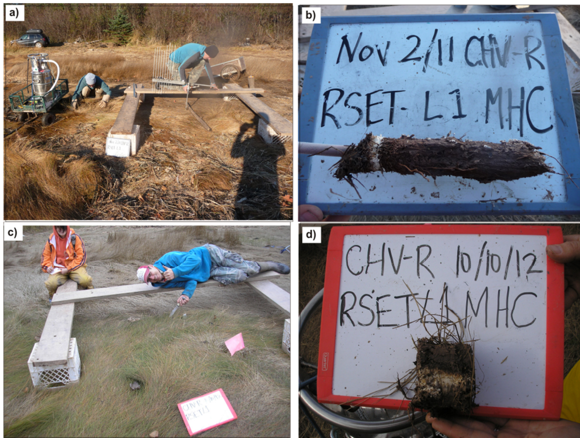
Figure 44 RSET-01 (LM) and associated marker horizon at CHV-R on a) Nov 2, 2011 and c) Oct 10, 2012. Note wrack material and debris in 2011.
