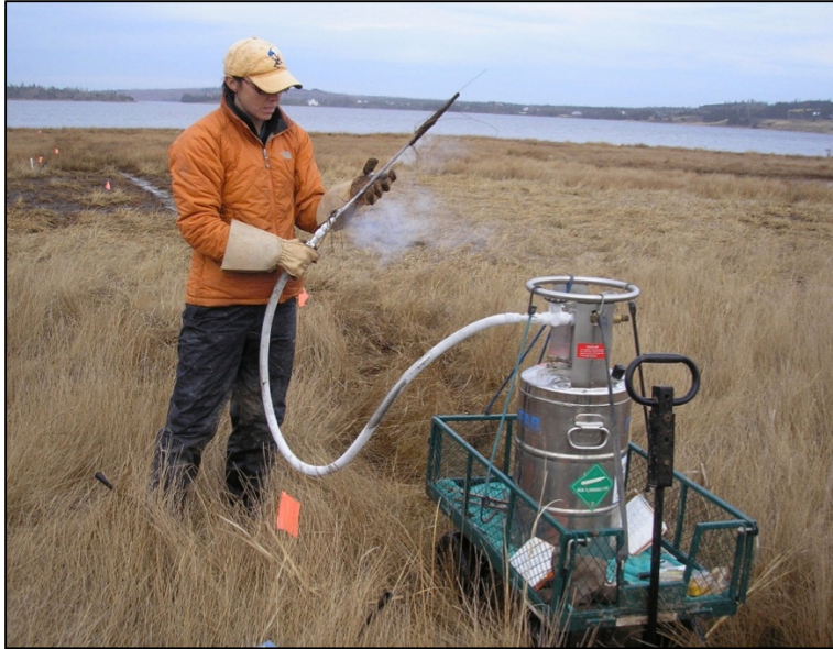
Figure 20: Marker horizon sampling with the cryogenic corer (with stainless steel tubing and copper “bullet”) at Lawrencetown Lake Reference Site. Photograph by B. Lemieux, December 2011.
