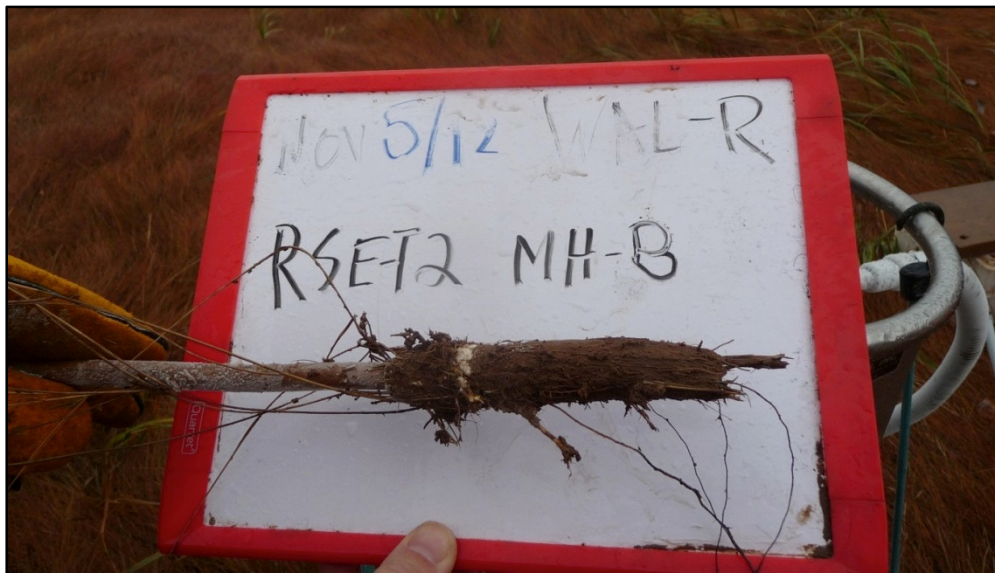
Figure 21: Core or "marsh-cicle" on bullet used for marker horizon calculations. Top of core is to the left. Photograph by B. Lemieux, November 12.
