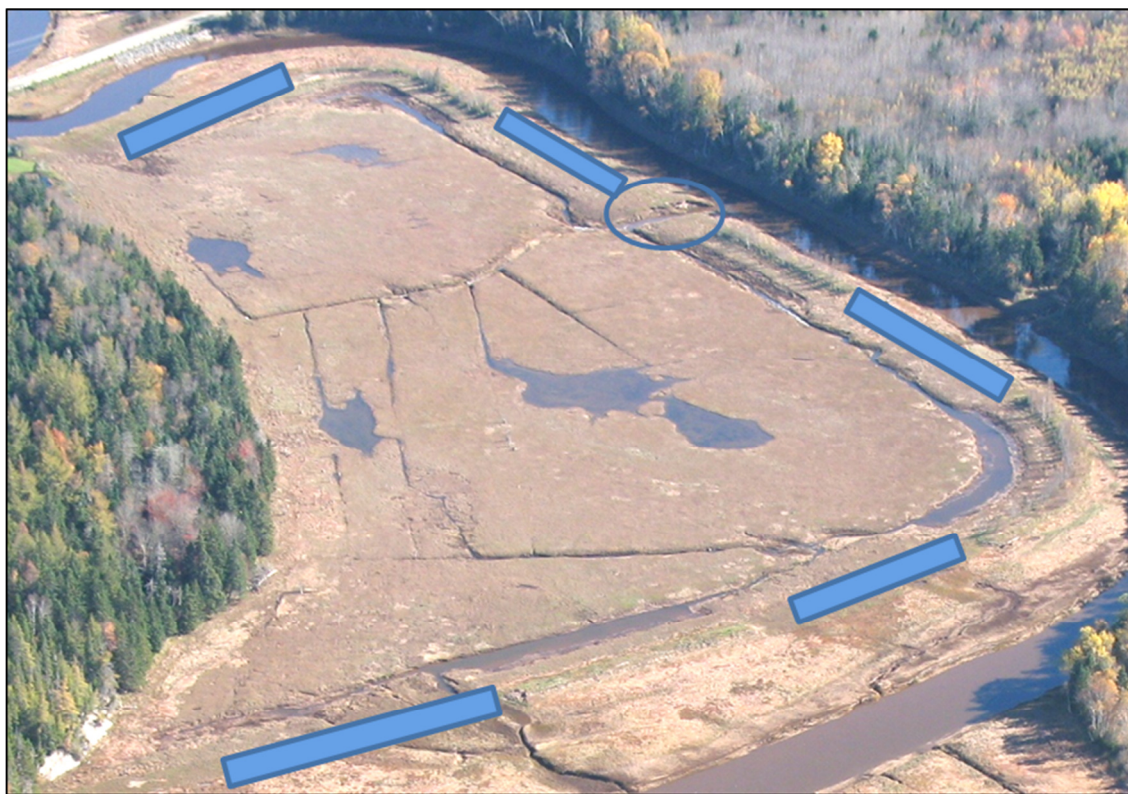
Figure 10: WAL 2012 showing the five breaches (solid blue), main channel (blue outline) and the channel network and pannes. Breaches are numbered 1 - 5 clockwise, starting from the top left corner. Aerial photography by Gaiamatics Solutions Inc. 28 October 2012.
